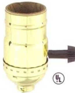
On/Off Turn knob Removable Turn-Knob Bushing Tapped 1/8IPS ( For 3/8" pipe) Rated 250W - 250V
